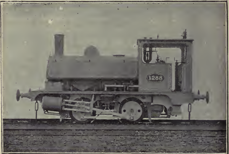
FIG. 120.—OIL-FIRED SADDLE TANK SHUNTING ENGINE, LANCASHIRE AND YORKSHIRE RAILWAY
