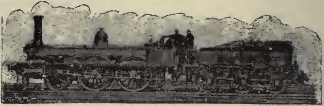
FIG. 35.—STEPHENSON'S "LONG-BOILER" GOODS ENGINE, EASTERN COUNTIES RAILWAY
