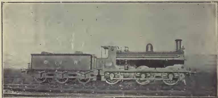
FIG. 123.—SIX-WHEELS-COUPLED CONDENSING ENGINE, CALEDONIAN
