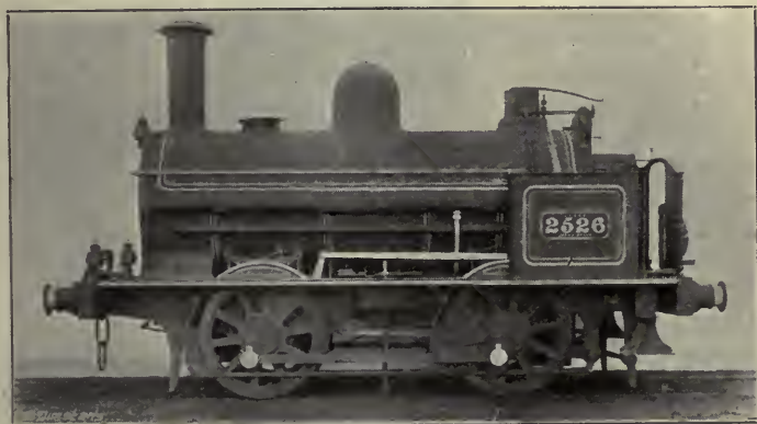
FIG. 118.—FOUR-WHEELS-COUPLED, SADDLE TANK ENGINE, LONDON AND NORTH WESTERN RAILWAY
