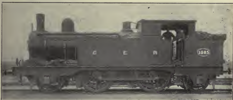
FIG. 123A.—A GREAT EASTERN RAILWAY "DOUBLE-ENDER," TANK ENGINE, FITTED WITH CONDENSING APPARATUS
