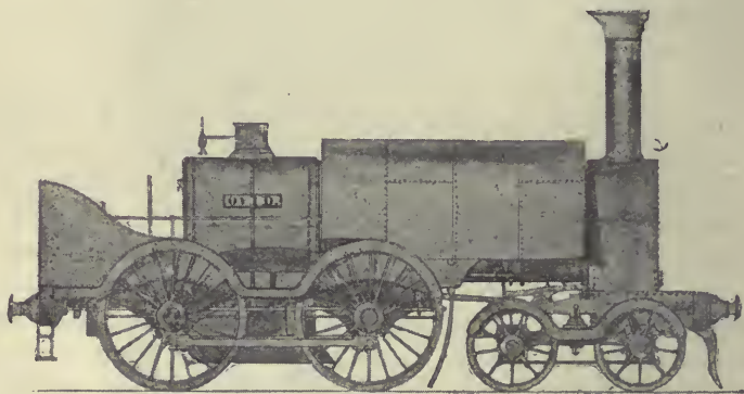
FIG. 71.—"OVID," A SOUTH DEVON RAILWAY SADDLE TANK ENGINE, WITH LEADING BOGIE
