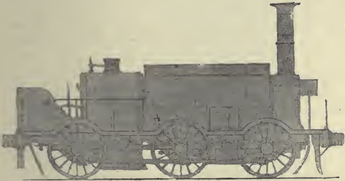
FIG. 72.—"PLATO," A SIX-COUPLED SADDLE TANK BANKING ENGINE, SOUTH DEVON RAILWAY
