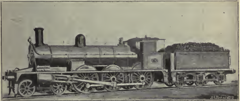
FIG. 141.—SIX-WHEELS-COUPLED BOGIE ENGINE, WITH OUTSIDE CYLINDERS, HIGHLAND RAILWAY
