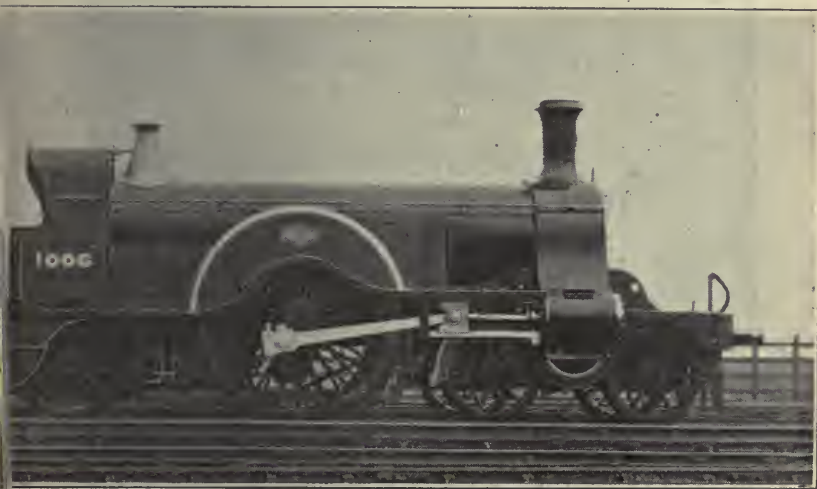
FIG 91.—3FT. 1IN. "SINGLE" EXPRESS ENGINE, GREAT NORTHERN RAILWAY
