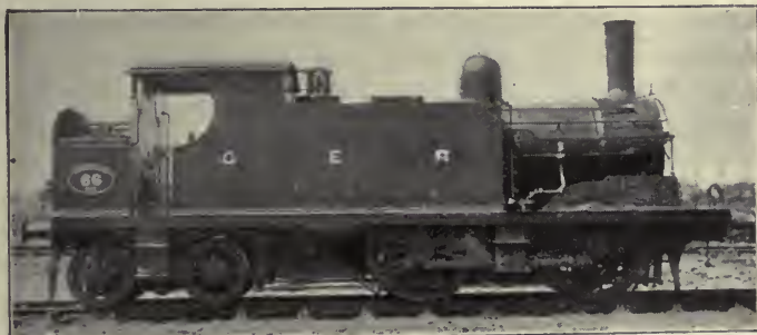
FIG. 126B.—GREAT EASTERN RAILWAY 4-COUPLED-IN-FRONT TANK ENGINE
